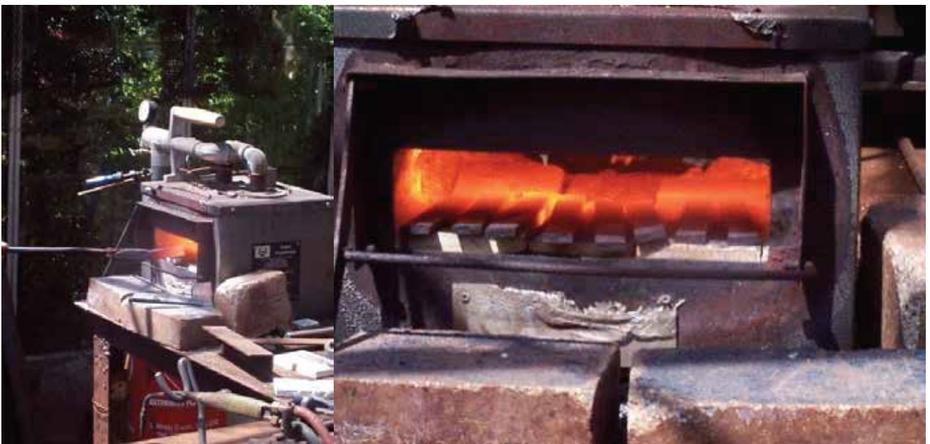
Producing Curls: Heating the metal strips
