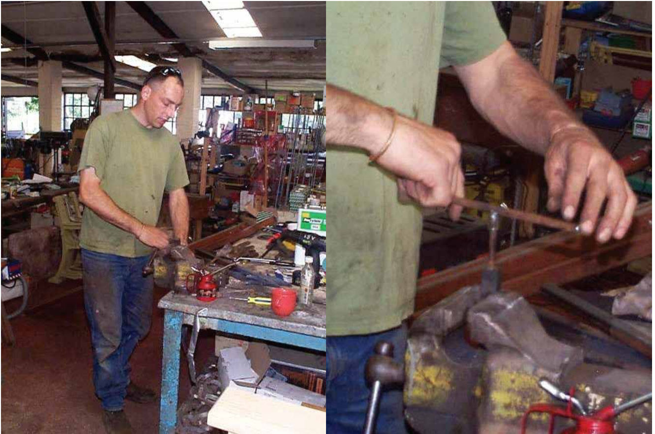
Tapping the arrow heads for assembly
